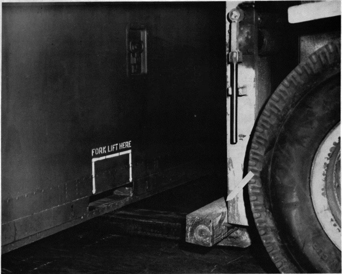
Figure 3. Dunnage placed on forks to avoid contact between the truck back plate and the side of the shelter.
