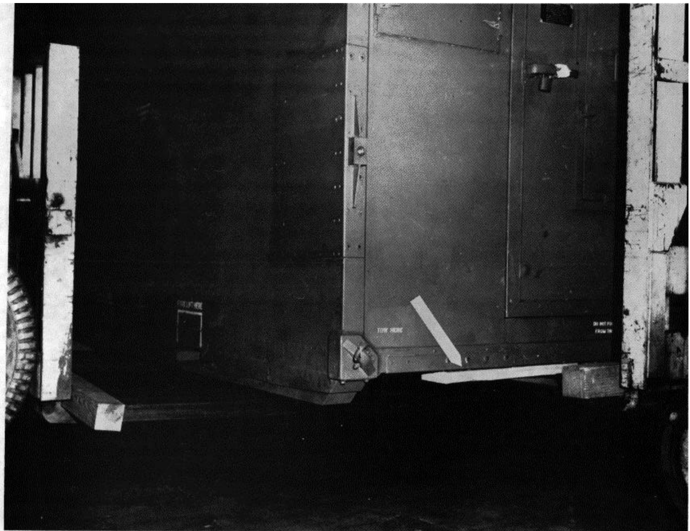
Figure 2. Arrows indicate placement of dunnage used to protect the bottom of shelter when raising one end.
